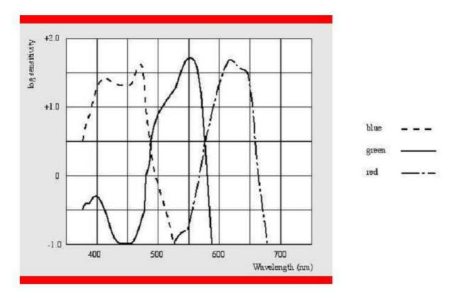
The curve refers to a density 1.0 above base fog. Sensitivity is reciprocal to the exposure expressed in  $mJ/m^2$ , required to produce that particular density.
